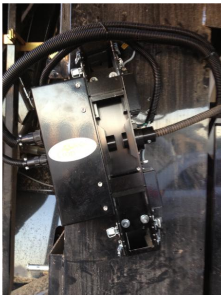
Figure 2. Remote Sampling Head shown as fitted to a clean grain elevator
