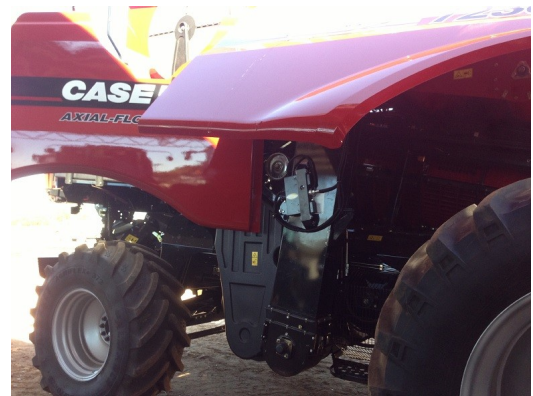
Fig 8 CropScan 3300H installed on a CASE combine
