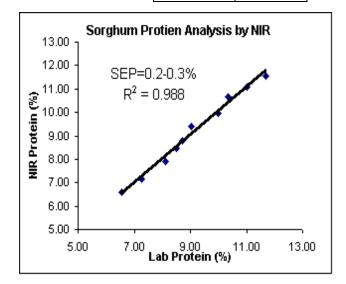
**Conclusion:** The above results show that the Cropscan 2000B whole grain analyser can be calibrated to measure the protein content of sorghum samples, which come from a wide variety of types and seasons. Slight adjustments to the pathlength and more data should lead to a robust calibration. Moisture analysis is already known to be successful in sorghum with prediction statistics of about 0.2%.
